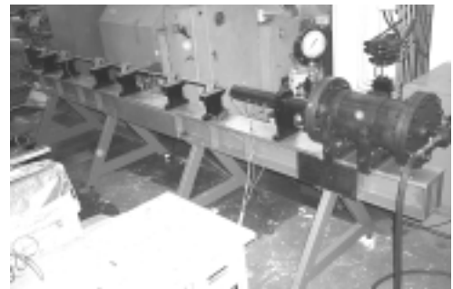
Fig. 2 Split Hopkinson pressure bar
