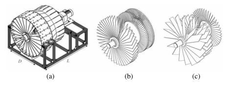
**Figure 3.** Experimentally designed jet engine models. (a) Isometric view of the overall engine structure, (b) rotating part of engine model A, (c) rotating part of engine model B.
