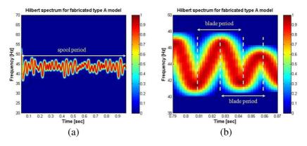
**Figure 4.** (a) Hilbert spectrum of the measured JEM signal of designed model A, (b) expanded Hilbert spectrum related to (a).
