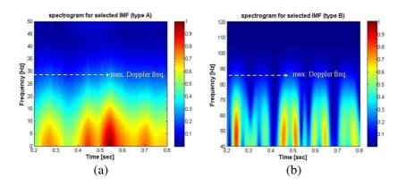
**Figure 7.** STFT spectrograms of the selected IMFs. (a) From designed engine model A, (b) from designed engine model B.
