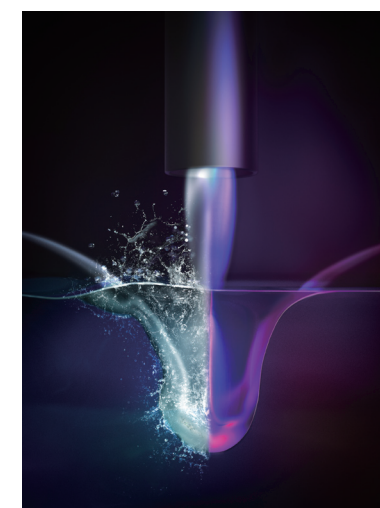
Figure 1. Illustration simulating the stabilization of a liquid surface through an ionized gas jet
