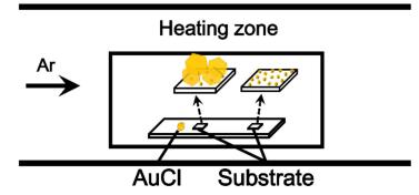
**Figure 1.** Schematic illustration of the vapor-phase synthesis of Au nanostructures (NSs) at low temperature. When the substrate was placed 15–20 mm away from AuCl, Au NPs were grown on the substrate. When the substrate was placed 3–5 mm away from AuCl, Au nanoplates were obtained on the substrate.
