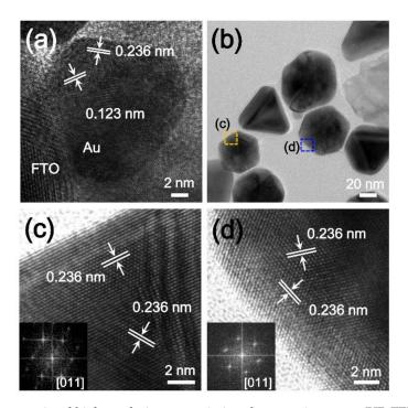
**Figure 4.** (a) Cross-sectional high-resolution transmission electron microscopy (HR-TEM) image of Au NPs on an FTO substrate. The Au NPs directly interfaced with the FTO substrate without any space; (b) TEM image of Au NPs detached from the FTO substrate; (c,d) HR-TEM images of Au NPs obtained from the (c) orange and (d) blue boxes of (b). Insets are fast Fourier transformation (FFT) patterns of the Au NPs.
