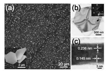
**Figure 5.** (a) SEM image of free-standing Au nanoplates synthesized on an FTO substrate. The inset is a magnified SEM image of the Au nanoplates; (b) TEM image and selected-area electron diffraction (SAED) pattern (inset) of the Au nanoparticles; and (c) cross-sectional HR-TEM image of the Au nanoplate.
