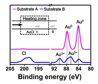
**Figure 2.** X-ray photoelectron spectroscopy (XPS) spectra obtained for two substrates placed in or out of the heating zone. Substrate A was positioned approximately 10 mm away from AuCl, and substrate B was positioned approximately 250 mm away from the precursor (inset). The binding energy peaks corresponding to Au<sup>0</sup> were measured on substrate A (magenta). Binding energy peaks corresponding to Au<sup>3+</sup> and Cl were measured on substrate B (blue).
