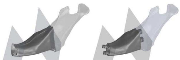
Figure 5: Different implant variants, left outer attachment to the residual bone, right inner attachment to spongy tissue
