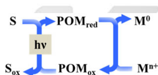
Figure 2. Polyoxometalate-assisted photocatalytic cycle for the reduction of a transition or noble metal ion to nanomaterials.
