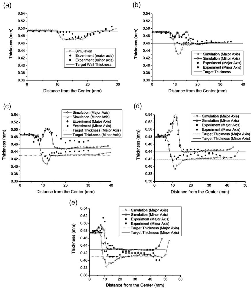
Fig. 14. Thickness distribution in each forming stage with the modified design: (a) stage 1; (b) stage 2; (c) stage 3; (d) stage 4; and (e) stage 5.
