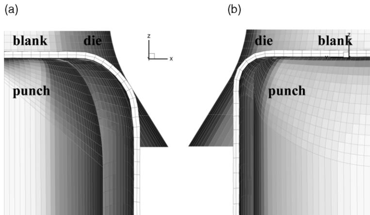
Fig. 15. Initial shape of tool positioning at stage 4 with the modified design: (a) minor axis; and (b) major axis.
