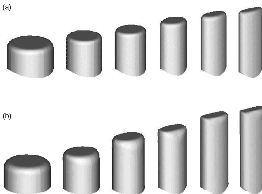
Fig. 12. Intermediate punch shapes in each forming stage: (a) initial design; and (b) modified design.
