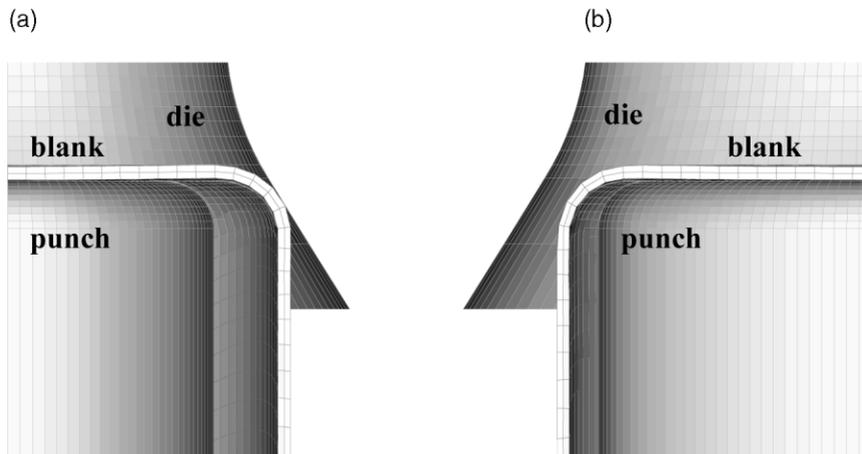
Fig. 8. Initial shape of tool positioning at stage 4 with the initial design: (a) minor axis; and (b) major axis.
