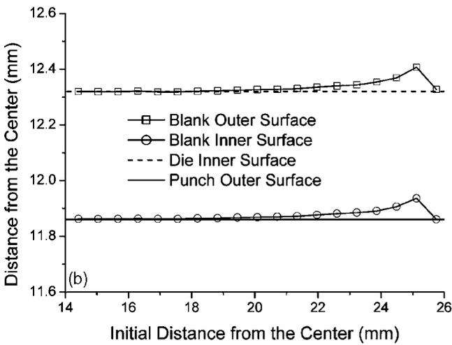
Fig. 7. Shape of the cup wall after the forming process: (a) stage 1 and (b) stage 2.
