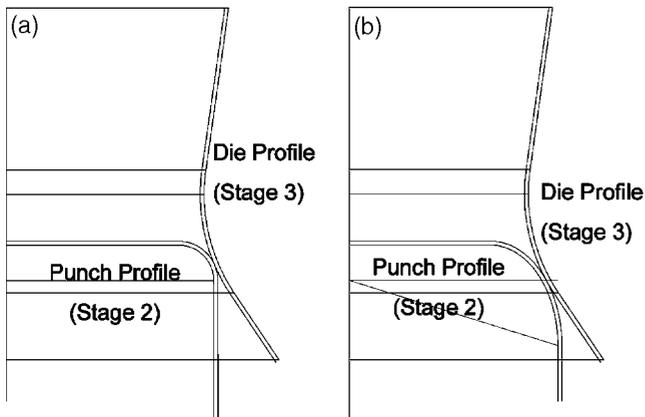
Fig. 10. Modifying procedure for the shoulder part of the punch at the minor axis at stage 2: (a) major axis; and (b) minor axis.
