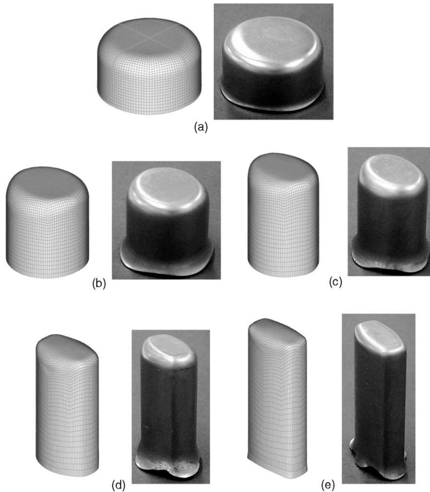
Fig. 13. Deformed shapes of the blank at each forming stage with the modified design: (a) stage 1; (b) stage 2; (c) stage 3; (d) stage 4; and (e) stage 5.
