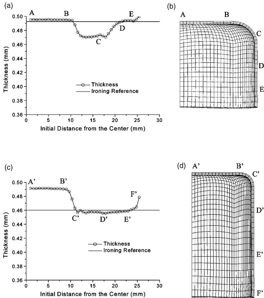
Fig. 6. Thickness distributions with the location of measuring points: (a) thickness distribution at the stage 1; (b) position of measuring points at the stage 1; (c) thickness distribution at the stage 2; and (d) position of measuring points at the stage 2.
