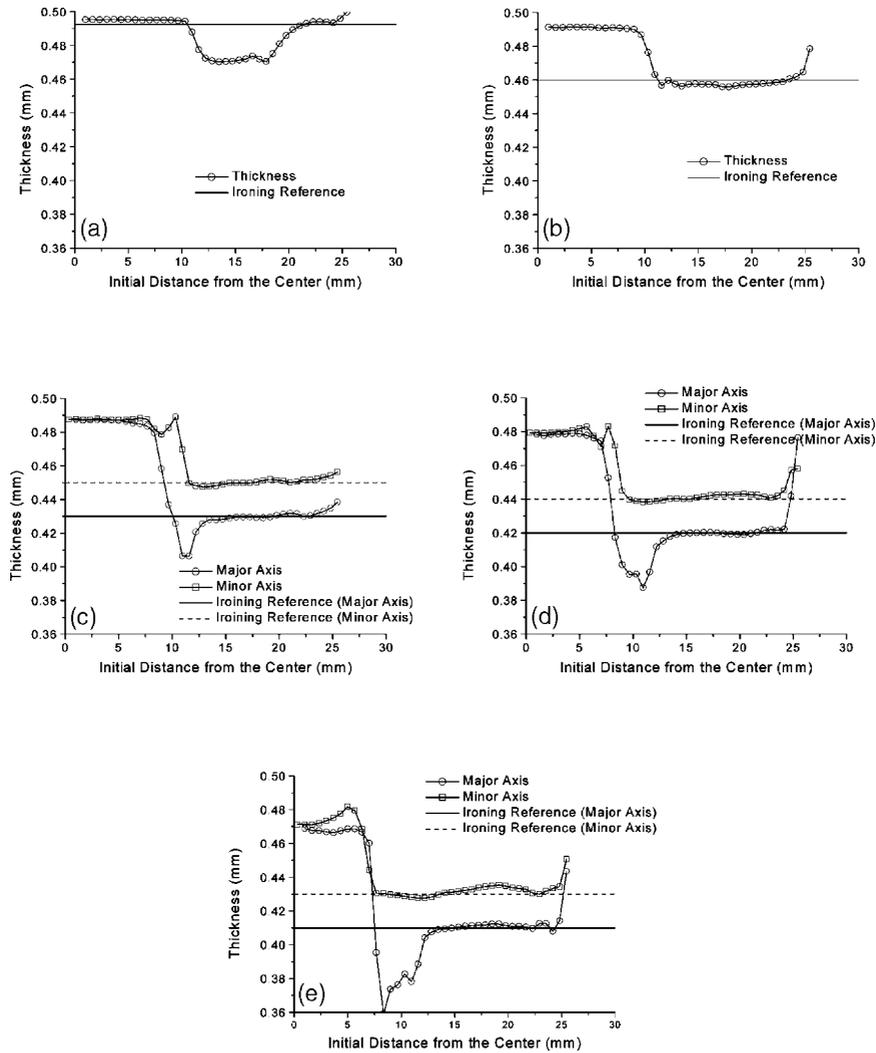
Fig. 5. Thickness distribution in each forming stage with the initial design: (a) stage 1; (b) stage 2; (c) stage 3; (d) stage 4; and (e) stage 5.
