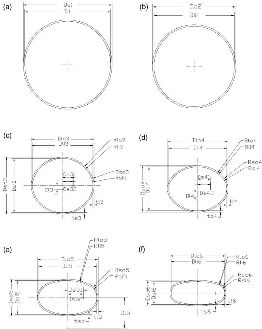
Fig. 1. Punch profiles at each forming stage in the initial design: (a) stage 1; (b) stage 2; (c) stage 3; (d) stage 5; and (e) stage 6.
