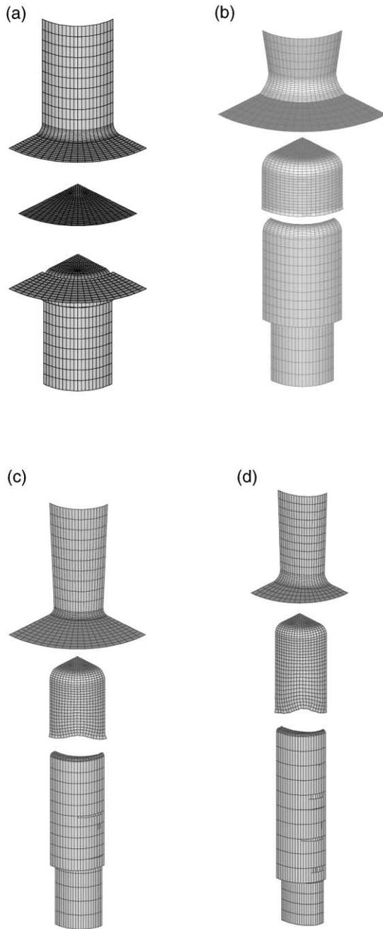
Fig. 3. Shape of tools and the blank in the initial design: (a) stage 1; (b) stage 2; (c) stage 3; and (d) stage 4.
