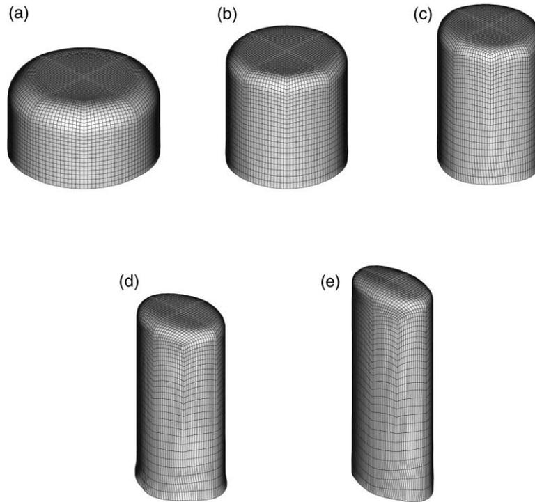
Fig. 4. Deformed shapes of the blank at each forming stage with the initial design: (a) stage 1; (b) stage 2; (c) stage 3; (d) stage 4; and (e) stage 5.
