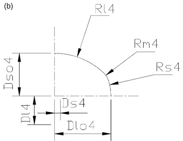
Fig. 9. Modification procedure for the cross section of the punch head at stage 4 (a quarter model) : (a) initial design; and (b) modified design.
