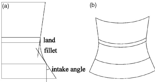
Fig. 11. Intake angle of the die with the modified design at stage 3: (a) side view; and (b) isometric view.
