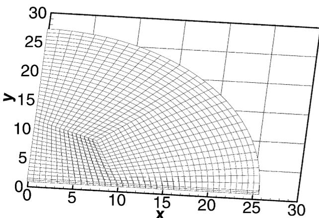
Fig. 2. Initial mesh system for the blank discretized by continuum elements.
