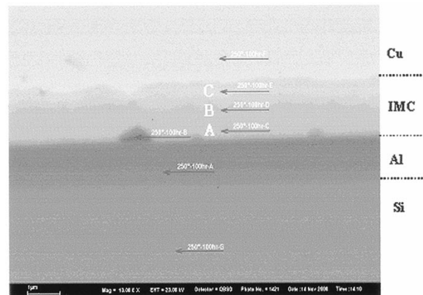
Fig. 3. SEM image of annealed Cu/Al sample at 250 °C for 100 h. EDS analysis was performed at A, B, and C points.
